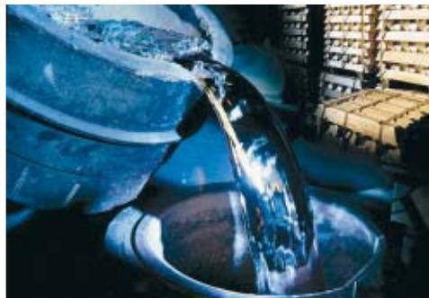
*Recycled aluminium poured into ingots for use in new applications*
